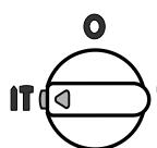
Position for hammer drilling
